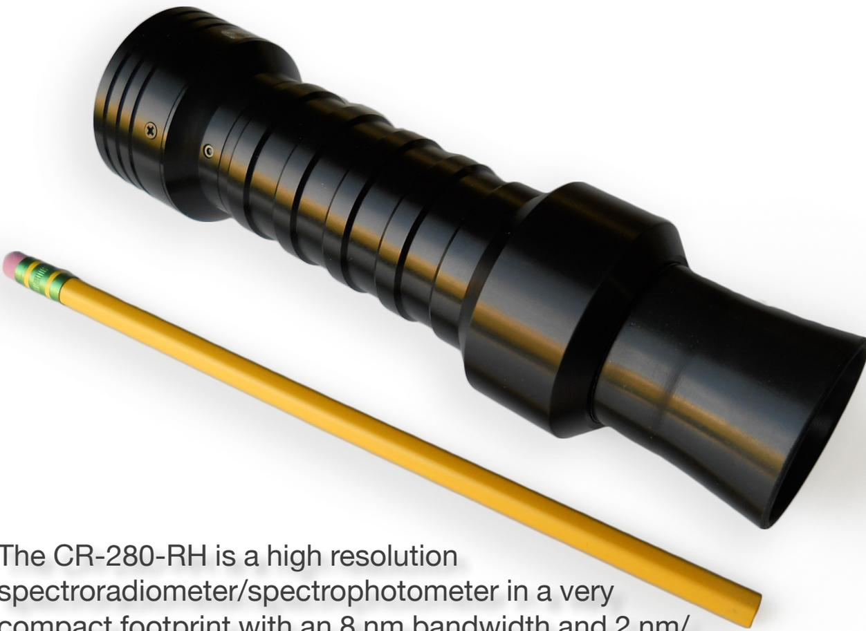
The CR-280-RH is a high resolution spectroradiometer/spectrophotometer in a very compact footprint with an 8 nm bandwidth and 2 nm/pixel resolution that excels in low-light, highly accurate VIS+NIR.
