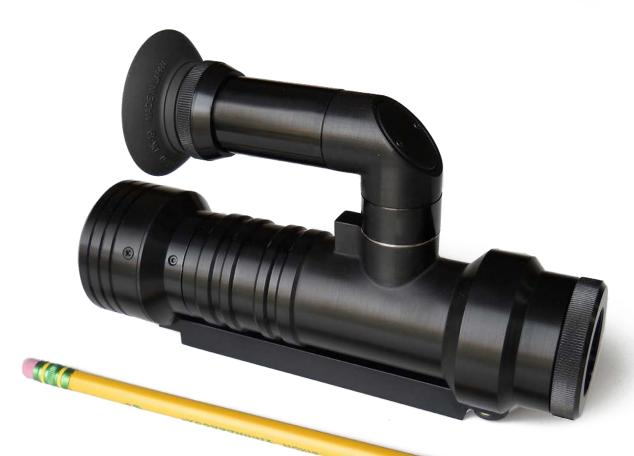
With the ability to capture data in less than 60 milliseconds, the CR-200 Tristimulus Colorimeter/ Photometer was designed for high-speed production line and Q.C. inspection, as well as product development.
