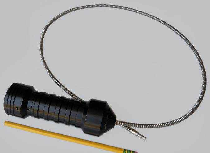
The CR-250-FP is a high resolution spectroradiometer in a very compact footprint with a 4 nm bandwidth and 1.6 nm/pixel resolution that excels in low-light, highly accurate wavelength and color measurements.
