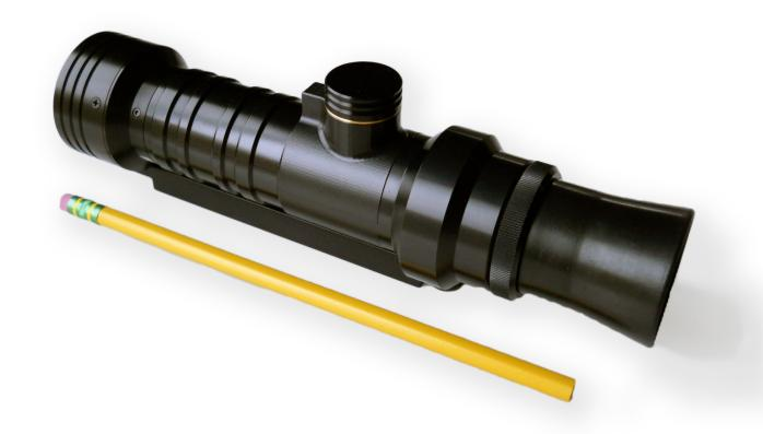
The CR-250 is a high resolution spectroradiometer in a very compact footprint with a 4 nm bandwidth and 1.6 nm/pixel resolution that excels in low-light, highly accurate wavelength and color measurements. It's ideal for measuring current and future display technologies as well as projectors including 6P projector technology.
